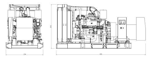
Drawing above for illustration purposes only, based on standard open power 400 Volt engine-generator set. Lengths may vary with other voltages. Do not use for installation design. See website for unit specific template drawings.
