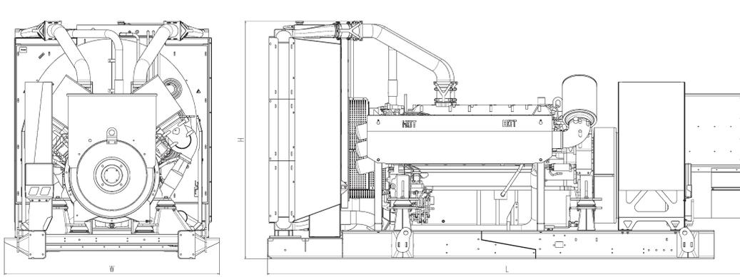
Drawing above for illustration purposes only, based on a standard open power 400 Volt engine-generator set. Lengths may vary with other voltages. Do not use for installation design. See website for unit specific template drawings.
